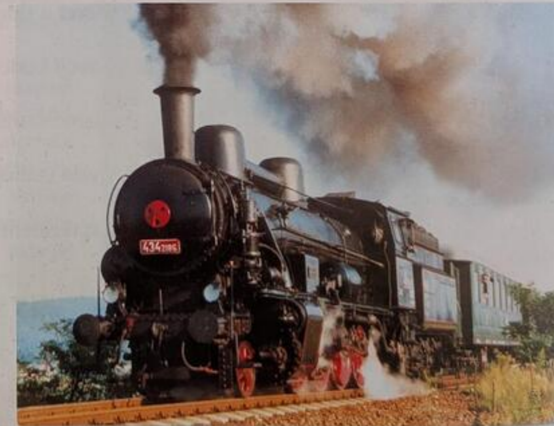
A steam locomotive manufactured for the Czechoslovak State Railways by the Českomoravská-Kolben-Daněk company. The locomotive weighed over 60 tons and reached a speed of 60 km/h.
