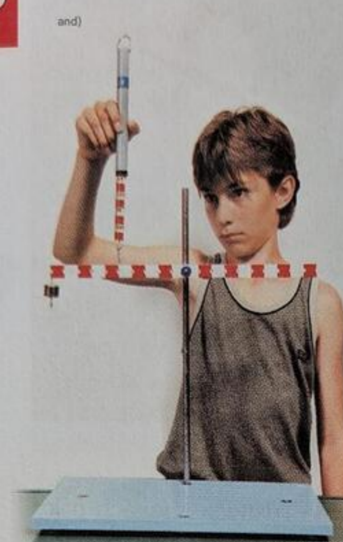
Fig. 1.87 Equilibrium position of a lever acted upon by two forces on the same side of the axis of rotation
